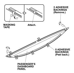
25. Align the passenger's dashboard panel and attach it as shown.
