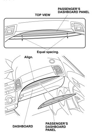
26. While applying light pressure against the passenger's dashboard panel, carefully remove the adhesive backings.
