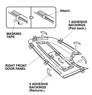
21. Align the right front door panel and attach it as shown.
