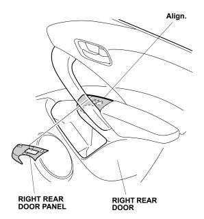
31. While applying light pressure against the right rear door panel, carefully remove the adhesive backings.
